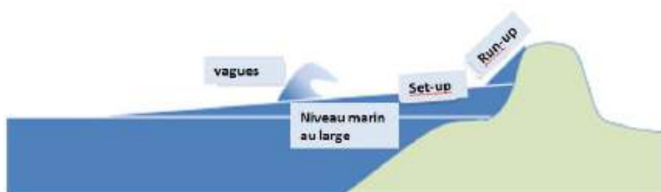
Figure 19 : principe du set-up
